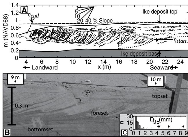
Deposit stratigraphy (Fig. 2) was characterized by sketching and photographing the trench wall, logging detailed stratigraphic sections at 2 m intervals, and collecting 2–4 sediment samples at each section for grain-size analysis.
